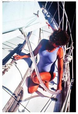
Moira's water catching awning has gutters along each side to duct water into the tanks. It can stay up in 30 knot winds and still catch rain. The 25mm diameter tubes make sure the water flows freely from the gutters into the tanks during heavy rains. We have taken on 500 litres in 30 minutes.
